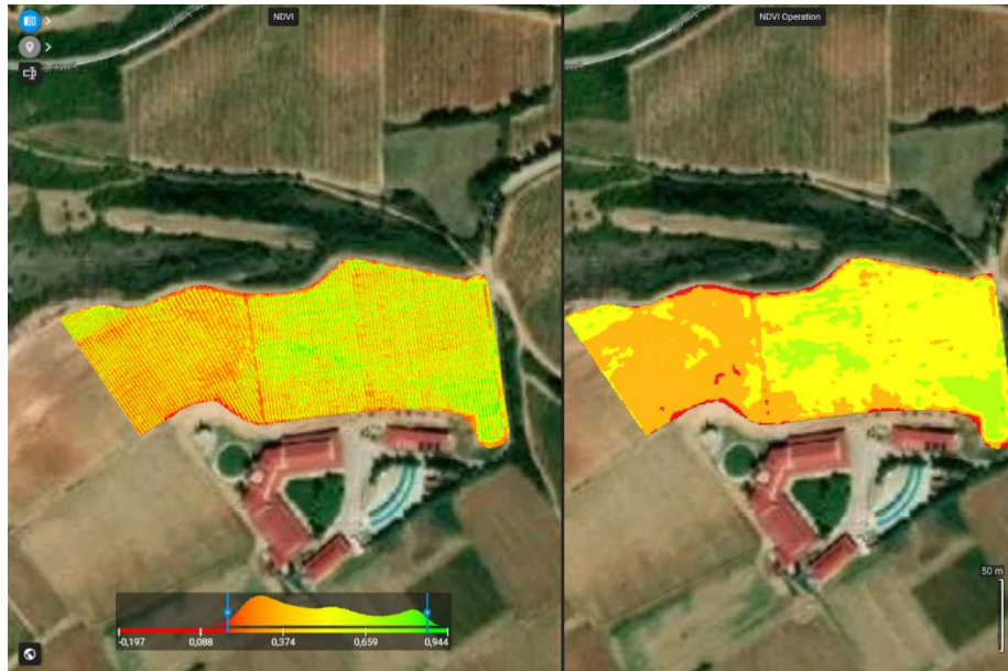
Figure 25: Indicative conversion of NDVI variability into prescription maps supporting precision input management.
